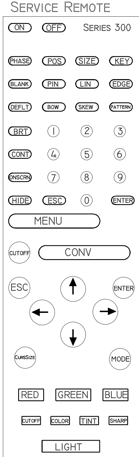
Figure 5-1. I/R Service Remote Control. Refer to Table 5-1 for description of key functions.
