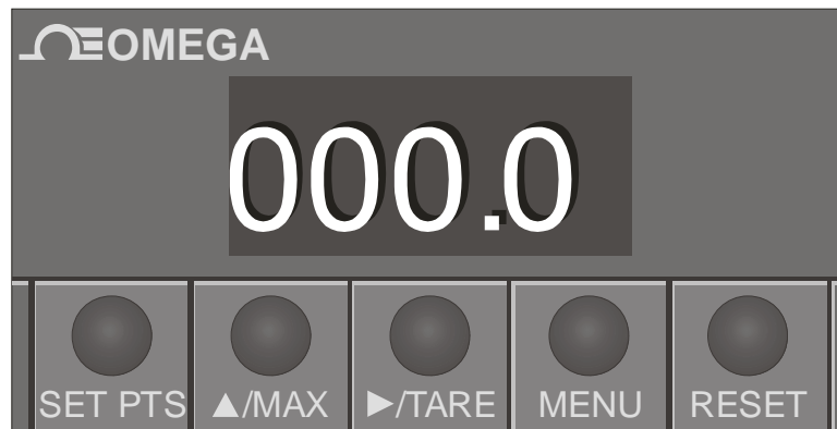
Figure 2-18 Air Pressure Meter for the Arc Lamp and ILA ® device HEPA air filters.
