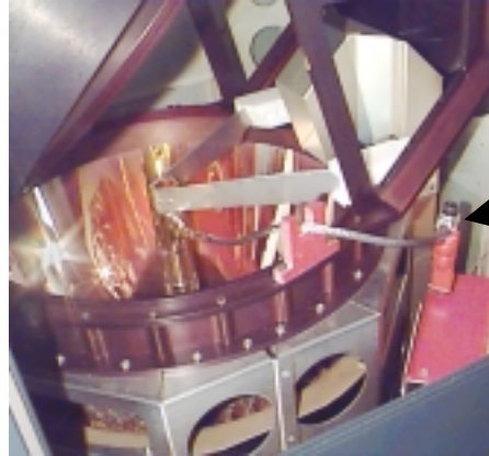
Figure 5-11 Arc Lamp Bulb installed with cable connected.
