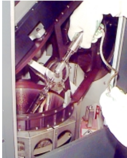
Figure 5-10 Insert the bulb into the bulb socket. Note that anode cable is at the top.
