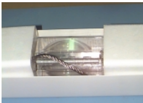
Figure 5-9 Remove bulb from container and place on padded table.
